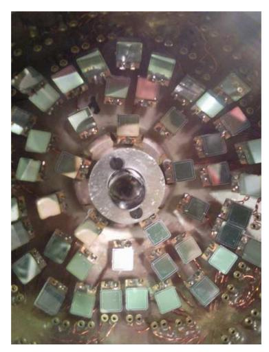
Figure 1: Backward hemisphere of the scattering chamber, with the degrader and PINdiode detectors visible.
