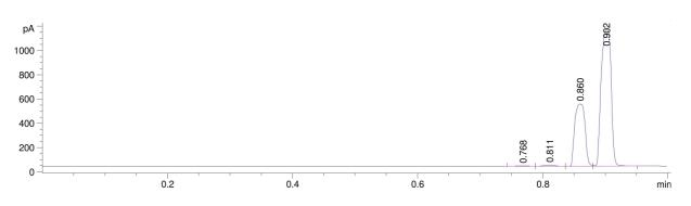
Figure 1: Gas-chromatographic separation of residual solvents. Signals, in order of appearance: methanol, ethanol, acetornitrile.
