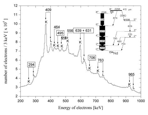
Figure 1: Total electron spectrum from the reaction:  ${}^{16}\text{O} + {}^{122}\text{Te} \rightarrow {}^{128}\text{Te}^*$ . The following lines may be recognised: decay of the isomeric state  $I^{\pi} = K^{\pi} = 8^{-}$  in  ${}^{134}\text{Nd}$  (text in rectangles), decay of  ${}^{134}\text{Pr}$  and decay of  ${}^{135}\text{Ce}$  (bold text).
