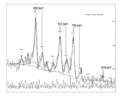
Figure 2: The summed "beam-off" electron spectrum in coincidence with the 294, 495 and 631 keV  $\gamma$ -ray transitions.
