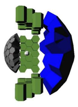
Figure 1: The setup for studying exotic neutron-deficient nuclei, consisting of a 1  $\Pi$  AGATA  $\gamma$  spectrometer, 1  $\Pi$  Neutron Wall, 1  $\Pi$  NEDA and 4  $\Pi$  DIAMANT charged particle detector.
