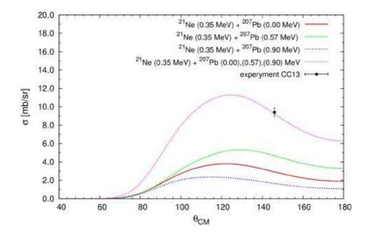
Figure 2: The cross section for the  ${}^{208}$ Pb( ${}^{20}$ Ne, ${}^{21}$ Ne) ${}^{207}$ Pb transfer. The red, green and blue curves correspond to calculations including the individual channels. The violet curve represent their sum.
