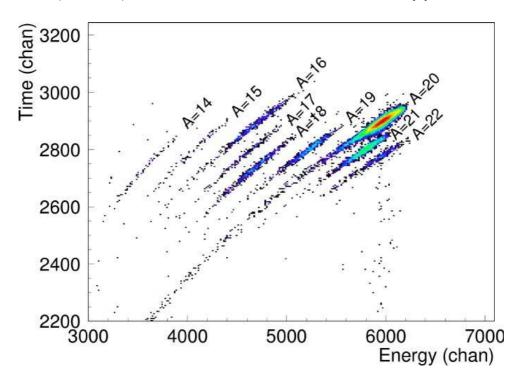
Figure 1: Typical two-dimensional E-TOF spectrum of the reaction products collected during one of the experimental runs.
