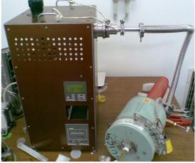
Figure 1: HPGe detector regeneration set-ups at HIL.
