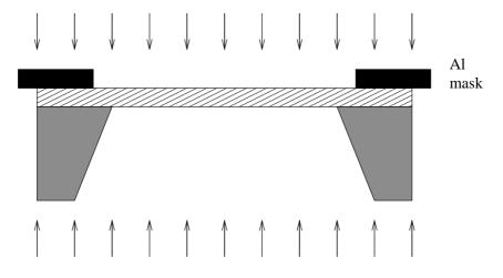
Al evaporation followed by long time baking of the Si detector
