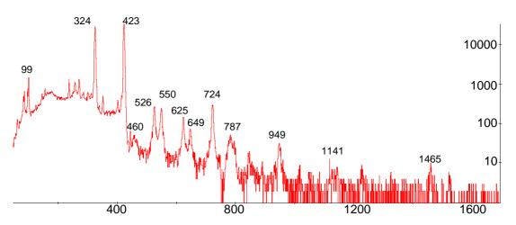
Figure 2: Gamma ray spectrum of <sup>107</sup>Ag Coulomb excited by a <sup>32</sup>S beam, summed over all HPGe and particle detectors. The  $\gamma$ -rays are in prompt coincidence with the scattered projectiles.
