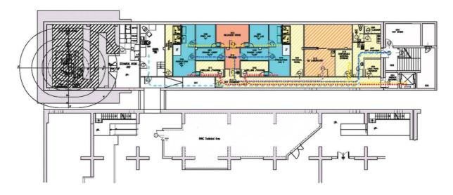
Figure 2: Layout of the RPRC. The proton/deuteron cyclotron and its control room is placed on the left part of the figure. Two independent production rooms are placed in the middle of the figure (the first one for the routine FDG production and the second one for other, also innovative, radiopharmaceuticals). The Quality Control room is placed in the right part of the figure (adapted from Refs. [2,4]).
