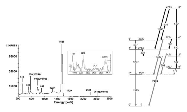
Figure 1: Left panel: a Doppler-corrected  $\gamma$ -ray spectrum observed in the  ${}^{42}\text{Ca} + {}^{208}\text{Pb}$ Coulomb excitation experiment. Right panel: The scheme of excited states in  ${}^{42}\text{Ca}$ . Transitions observed in the current Coulomb excitation experiment are marked in grey.
