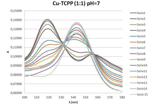
Figure 1: Kinetic spectra of Cu-Tetracaroboxyphenyloporphyrin formation.
