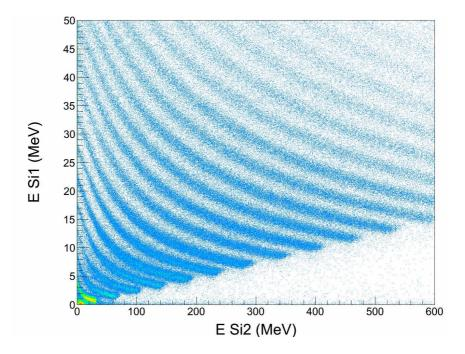
Figure 2:  $E-\Delta E$  scatter plot obtained using the  $E-\Delta E$  telescope consisting of 21  $\mu m \Delta E$  detectors with an active area of 20 \* 20 mm<sup>2</sup> and a 500  $\mu m E$  detector.
