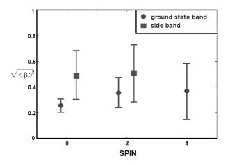
Figure 2: Preliminary values of the overall quadrupole deformation parameters  $\sqrt{\langle \beta^2 \rangle}$  calculated for 0<sup>+</sup>, 2<sup>+</sup> states in both ground state and side bands, as well as that of the 4<sup>+</sup><sub>1</sub> state in <sup>42</sup>Ca.
