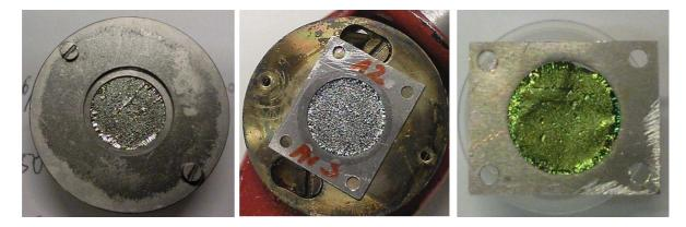
Figure 3: Left: the Ni target in the holder of the sputtering device (from the Ni side). Centre: the circle of the nickel (darker grey ring) on the frame guarantees the nickel contact with the frame to facilitate the heat transfer from the target material. Right: view of the target from the PIF side.
