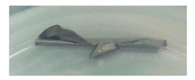
Figure 1: Ni foil made by sputtering on the Cu backing after etching the backing.
