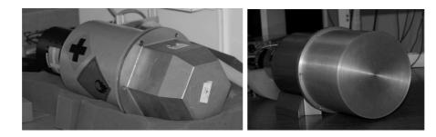
Figure 1: Neutron detectors used in the test measurements – the NORDBALL H10 detector evaluated in Uppsala (left) and a cylindrical detector tested in Warsaw (right).
