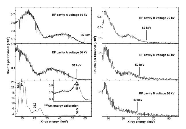
Figure 1: X-ray spectra for the two RF-cavities for three different voltmeter voltages (60, 66 and 72 kV) and the 15 MHz RF frequency. The  $^{241}$ Am X-ray calibration spectrum is also shown. The measured voltages are marked in the plots.
