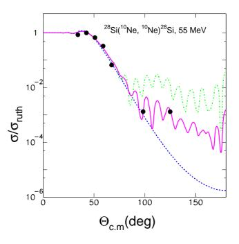
Figure 1: Elastic scattering data for  ${}^{20}\text{Ne}+{}^{28}\text{Si}$  at bombarding energy of 55 MeV are compared with coupled channel calculations. Results without coupling are denoted with the dashed curve while results with coupling with the dot-dashed and solid curves (spectroscopic factor equal to 1 and to 0.5, respectively).
