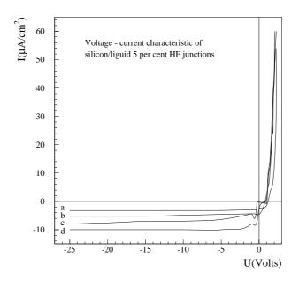
Figure 2: Voltage-current characteristics of silicon/liquid 5% HF junctions. (a) High resistivity silicon. Float zone. Tewa. (b) High resistivity silicon. Float zone. Topsil. Open circuit voltage 0.83 V. (c) High resistivity silicon epitaxial n<sup>+</sup>-n. ITME. Open circuit voltage 0.63 V. (d) High resistivity silicon epitaxial n<sup>+</sup>-n. ITME. Open circuit voltage 0.68 V. All voltages were measured with light illumination of junctions.
