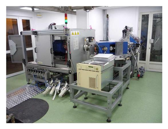
Figure 2: New ECR ion source with the horizontal part of injection line
