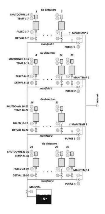
Figure 1: Scheme of the EAGLE  $\mathrm{LN}_2$  filling installation.
