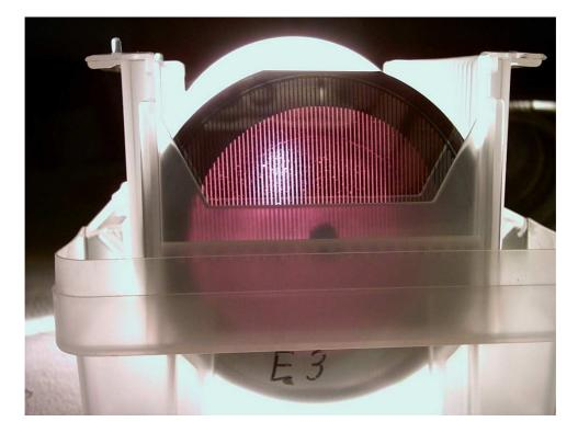
Figure 1: Four inch wafer with 7.3  $\mu$ m thin silicon membrane supported by a thick 400  $\mu$ m silicon n<sup>+</sup> substrate ring. The detector strips are visible in light illuminating the wafer from the back side.
