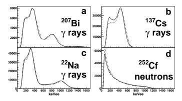
Figure 2: Experimental (solid line) and simulated (dotted) spectra obtained with the NORDBALL detector for  $\gamma$ -ray sources <sup>22</sup>Na (a), <sup>207</sup>Bi (b) and <sup>137</sup>Cs (c); as well with the cylindrical detector for neutrons emitted by the <sup>252</sup>Cf source (d). Neutrons were distinguished from  $\gamma$  rays using the charge-comparison method.
