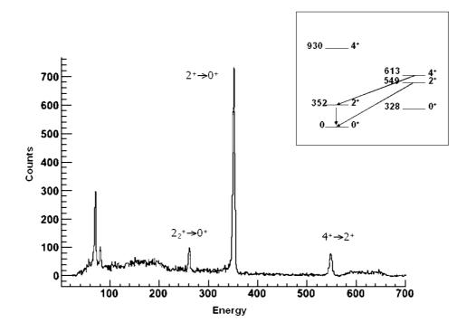
Figure 1: Total Doppler-corrected gamma-ray spectrum obtained for <sup>182</sup>Hg.
