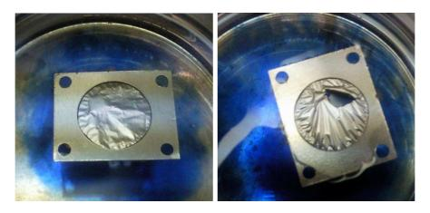
Figure 2: Ni foils prepared on the Cu backing during etching process
