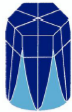
MINIBALL triple-clusters with 6 and 12 fold segmentation
