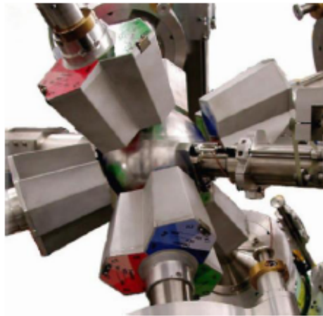
MINIBALL triple-clusters with 6 and 12 fold segmentation
