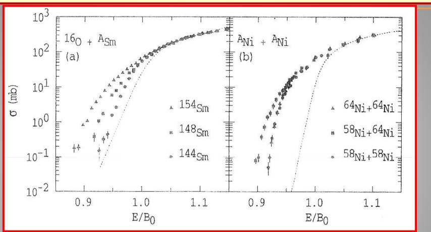
•Fusion excitation functions for <sup>16</sup>O on Sm isotopes show a marked increase of cross section with increasing mass and deformation.
