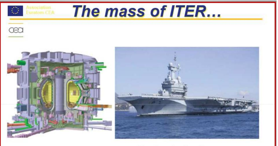
ITER Machine mass: ~23000 t 28 m diameter x 29 m tall Charles de Gaulle mass: ~38000 t (empty) 856 ft (261 m) long (Commissioned 2001)
