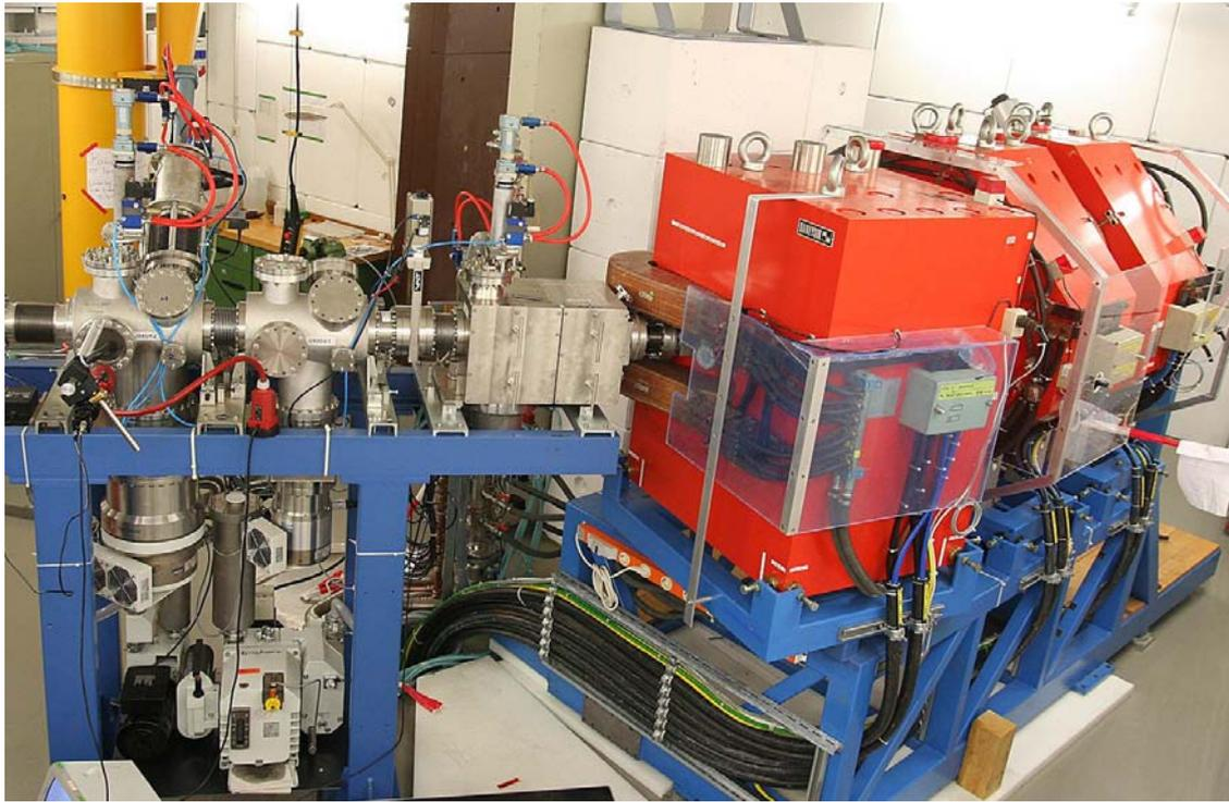
Fig. 2: View (from left to right, beam direction) of two diagnosis chambers, the target chamber (center) and the TASCA magnets.
