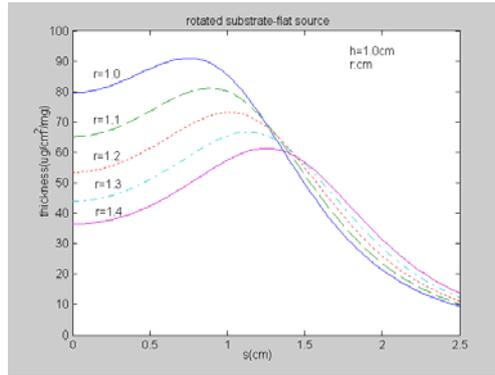
Fig.2. Theoretical film thickness distributions for a source-to-substrate distance  $h=1.0\text{cm}$ .
