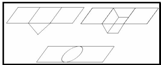
Figure 1 - Ta boats of 0.2mm thick pure Ta sheet, home made by cutting and modelling properly.
