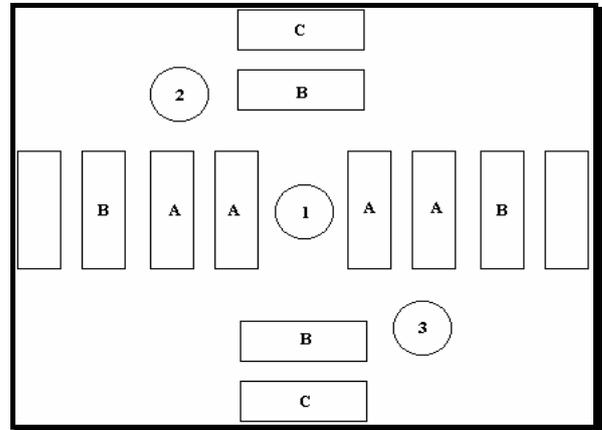
Figure 2 - Schematic view of the substrate holder. The circles numbered 1, 2 and 3 are the sites where the reference glass squares are loaded.
